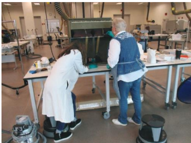
Cynthia Blechl (on the right) is cleaning the bellows using deionized water and cotton-tipped applicators in our state of the art facility. April Berry (on the left) is adhering the loose strap to the back of the pedal.
